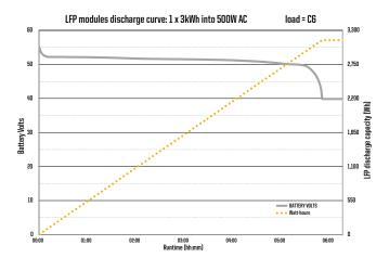
Tests reflect off grid usage. Data is based on Australian QA test programming. Results may vary with inverter efficiency and loom loss. Test load at 240V AC .
